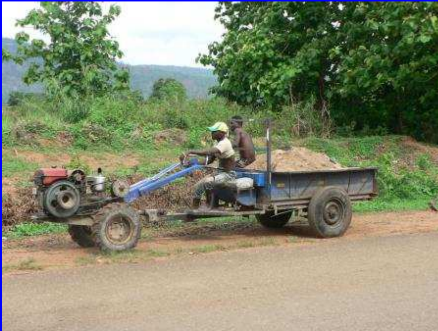
A power tiller mounted with a small trailer for rural transportation in Hohoe
