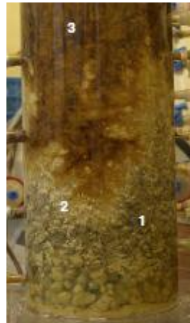
Column experiment of limestone-DAS
