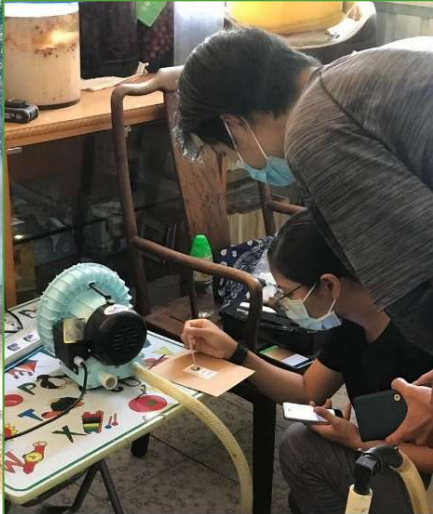
Use of micro Biometer Measuring microorganism concentration in the compost tea and the respective fungi-bacteria ratio
