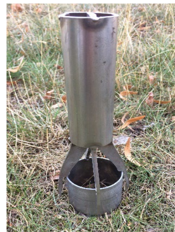
Figure 20: Core rings for the determination of the bulk density of the fine soil
