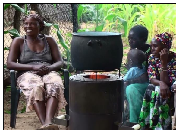
Figure 9: Namibian research partners work also on technologies that are adapted to the needs and habits of the people. Here a TLUD stove that produces biochar as well as heat for cooking. ©Dr. Ibo Zimmermann
